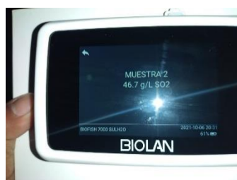
Figure 18: BIO7000 showing the result of sulphite measurement on field
