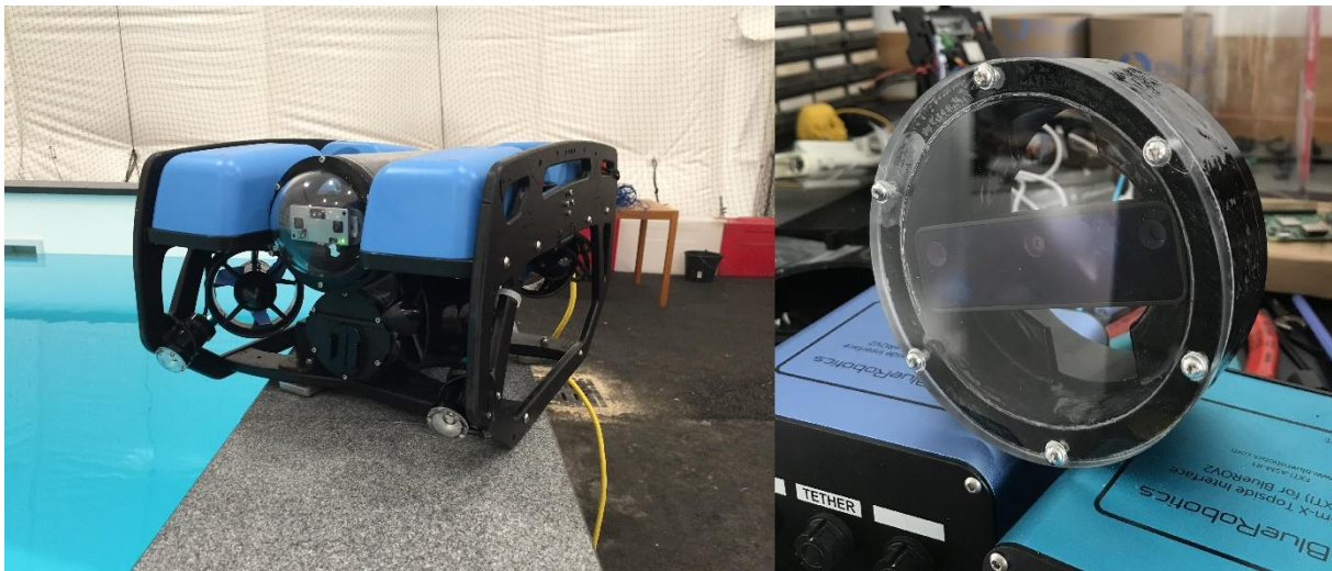
Figure 1: Left: Prototype BlueROV2/MyntEye D1200 Nose Camera Integration with Bubbledome. Right: Final Oak D Lite Nose Camera Integration with Flat Glass Plate.
