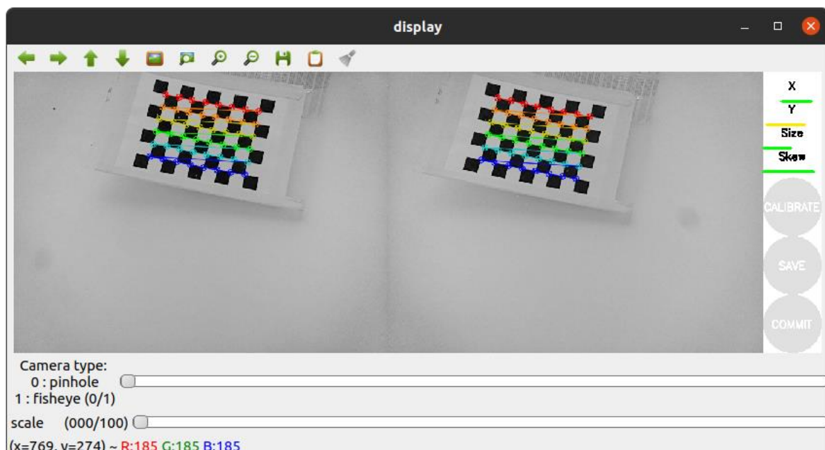
Figure 4: A sample used in the underwater stereo calibration process. Corresponding corners of the checkerboard pattern are matched between the left and right cameras. The calculated transformation is used to estimate intrinsic, extrinsic and distortion information about each camera
